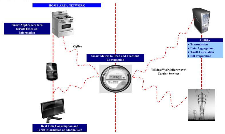
Smart Meter-the communication hub for smart grid
